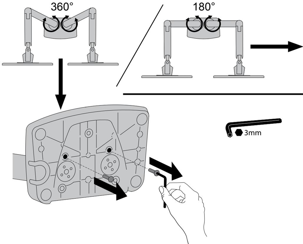
How to replace rotation stop screws (Arms must be straight up)
